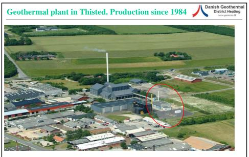
Established as a pilot plant in 1984 and later expanded to extract up to 7 MW heat from 200 m3/h of 44 °C, 15 % saline geothermal water from Gassum sandstone at 1.25 km depth.
