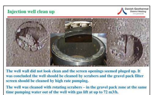
Thereafter the production pump was moved to the injection well and a cleanup pumping was made 10-13. October at rates up to 350 m3/h. Drawdown indicates an injection capacity exceeding 350 m3/h at the injection temperature viscosity.
